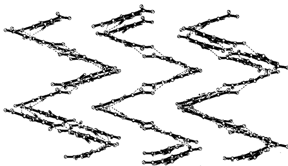
FIGURE 6 Edge-on view of buckled anionic sheets in 2 .
